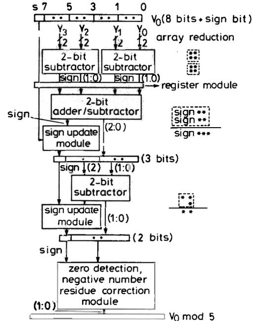
**Fig. 3** Schematic diagram of  $V_0 \bmod 5$  unit where  $V_0$  is an 8-bit number
