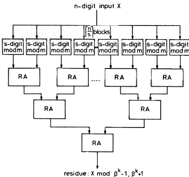
Fig. 2 Logical structure of the partition method for computing  $X \bmod \beta^k - 1, \beta^k + 1$
